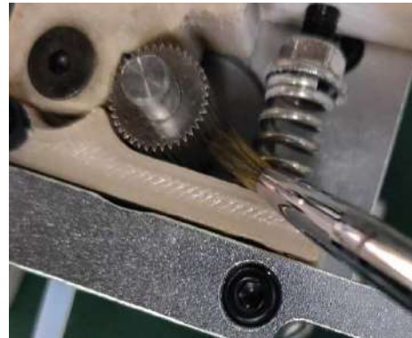
Clean the extruded tooth surface with a brush
